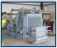
450 HP Diesel 4-Stage Pump, 6" x 6" with flowmeter Maximum Flow Rate - 1200 GPM Maximum Pressure (at pack-out) - 800 PSI
