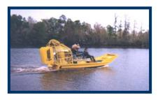
Our amphibious airboats and arsenal of motorboats allow our crews to access the most remote pipeline locations. This equipment allows us to set AGMs and track pigs in swamps and other bodies of water.
